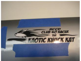
\*After the transfer paper is completely removed and the vinyl decal is in place on the plane, gently press on the decal with a dry soft cloth to insure the decal is completely dry, and stuck to the plane.
